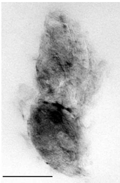
Fig. 1 TEM images of a graphite particle (scale: 100 nm)
